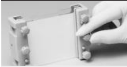
Fig 2.11. Slide the sandwich into the clamp assembly with the notched plate facing inward and secure by tightening screws.
