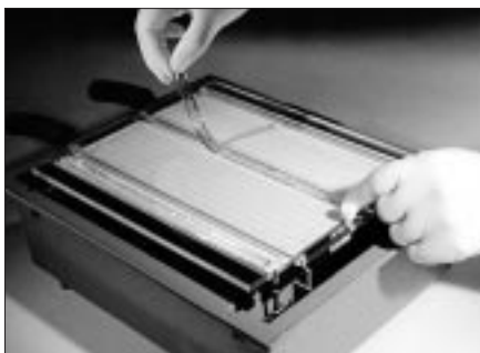
Fig 2.24b. Place the appropriate colour-coded buffer strips along the anodic and cathodic ends of the gel.
