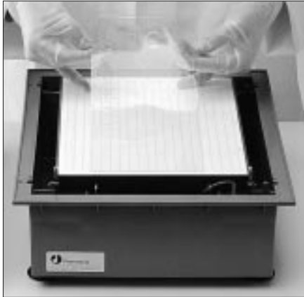
Fig 2.23. Placing the gel on the Multiphor II cooling plate.
