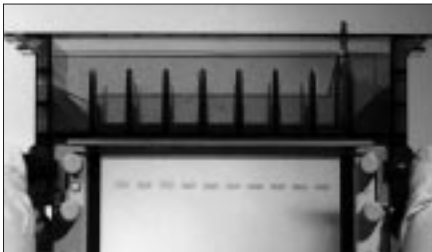
Fig 2.8. Locking the upper buffer chamber in place.
