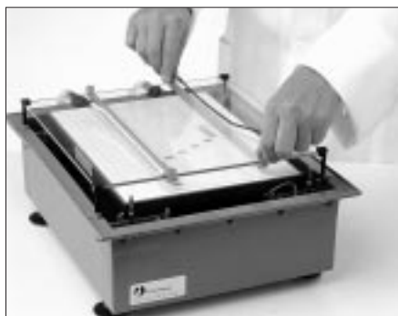
Fig 3.9c. Position the electrode holder over the electrode strip.
