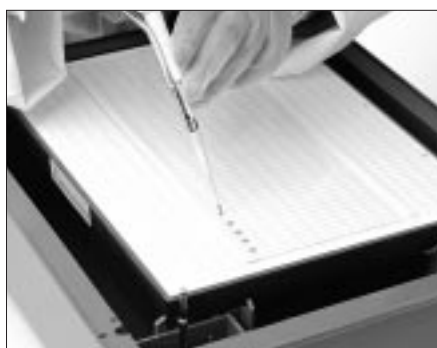
Fig 3.9b. Pipetting samples into applicator strip wells.
