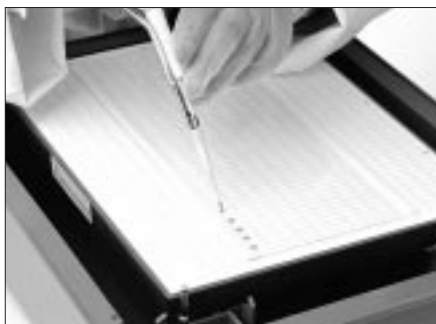
Fig 3.6b. Pipetting samples into the applicator strip wells.
