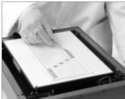
Fig 3.9a. Placing sample application pieces across the gel.
