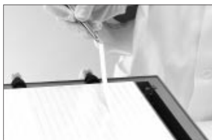
Fig 3.5. Applying an electrode strip near the anode.
