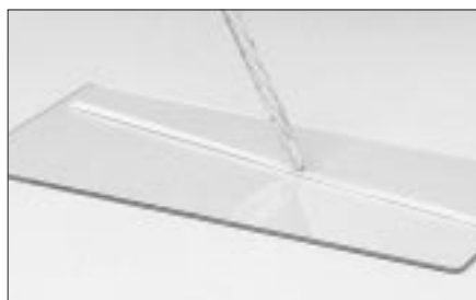
Fig 3.4. Soak the electrode strip in analyte or catholyte.
