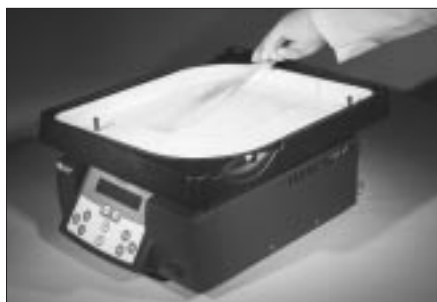
Fig 4.1. Processor Plus with large gel staining tray.
