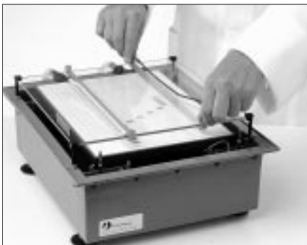
Fig 3.9c. Position the electrode holder over the electrode strip.
