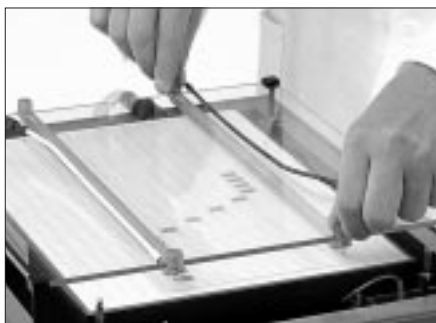
Fig 3.7. Positioning the electrode holder over the electrode strip.
