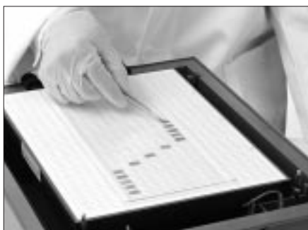
Fig 3.6a. Placing sample application pieces across the gel.
