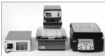
Fig 2.22. Multiphor II Flatbed Electrophoresis System.
