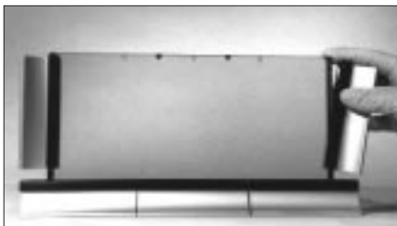
Fig 3.11. Clamp together the glass plates of the reswelling cassette.
