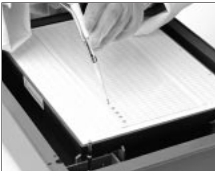
Fig 3.9b. Pipetting samples into applicator strip wells.
